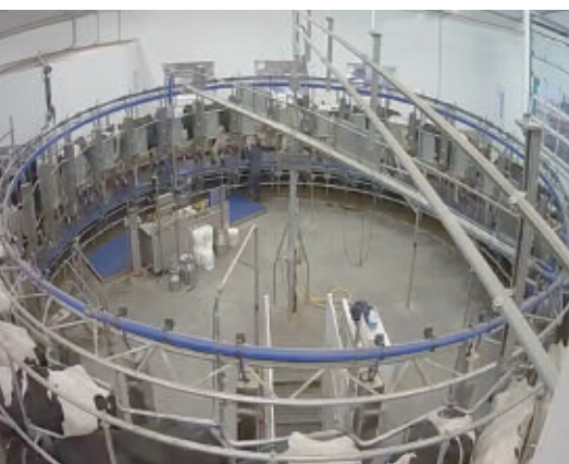
The new barn at Ferme Champagne is equipped with a 30-cow carousel and the cows are milked two or three times a day, depending on their stage of lactation.
