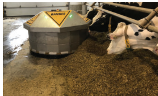
Automated feed pushers improve feeding and ensure a calm environment for cows.
